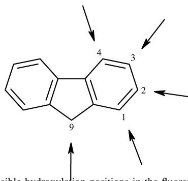
Fig. 1. Possible hydroxylation positions in the fluorene molecule.
