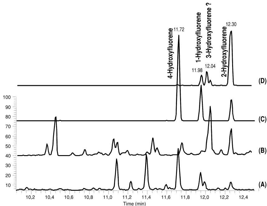
Fig. 8. GC–MS analysis after SPME sampling and derivatization with BSTFA: scanned acquisition as described in Section 2.4. (A) TIC and (C) mass trace 239 of a buffer solution, spiked with 1-, 2-, 4-, and 9-hydroxyfluorene at the upper working range. (B) TIC and (D) mass trace 239 of a urine sample, obtained from a worker occupationally exposed to PAHs.
