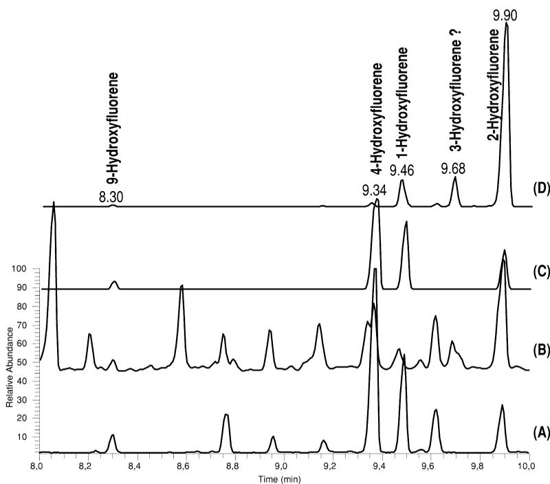
Fig. 2. GC–MS analysis after SPME sampling and derivatization with BSTFA: scanned acquisition as described in Section 2.4. (A) TIC and (C) mass trace 254 of a buffer solution, spiked with 1-, 2-, 4-, and 9-hydroxyfluorene at the upper working range. (B) TIC and (D) mass trace 239 of a urine sample, obtained from a worker occupationally exposed to PAHs.
