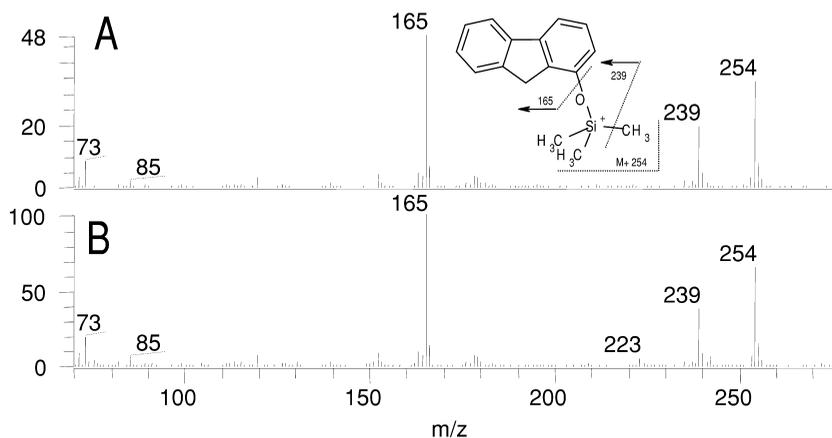
Fig. 3. Mass spectra of 1-hydroxyfluorene TMS ether after SPME and derivatization with BSTFA: (A) standard and (B) urine sample.
