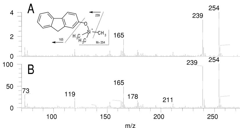
Fig. 4. Mass spectra of 2-hydroxyfluorene TMS ether after SPME and derivatization with BSTFA: (A) standard and (B) urine sample.
